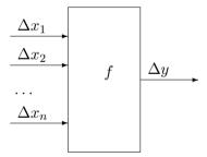
Traditionally, in engineering and science, we assume that we know the joint probability distribution for  $\Delta x_i$ . Usually, it is assumed that these measurement errors are independent and normally distributed, with 0 mean and known standard deviations; however, there are are also known ways of handling possible dependence and non-Gaussian (non-normal) distributions.
