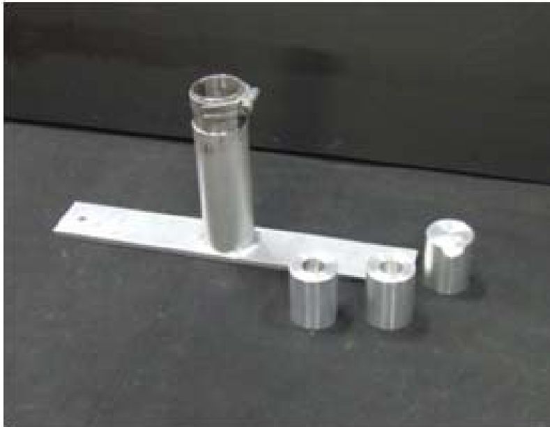
Fig.2 Rig with sockets
