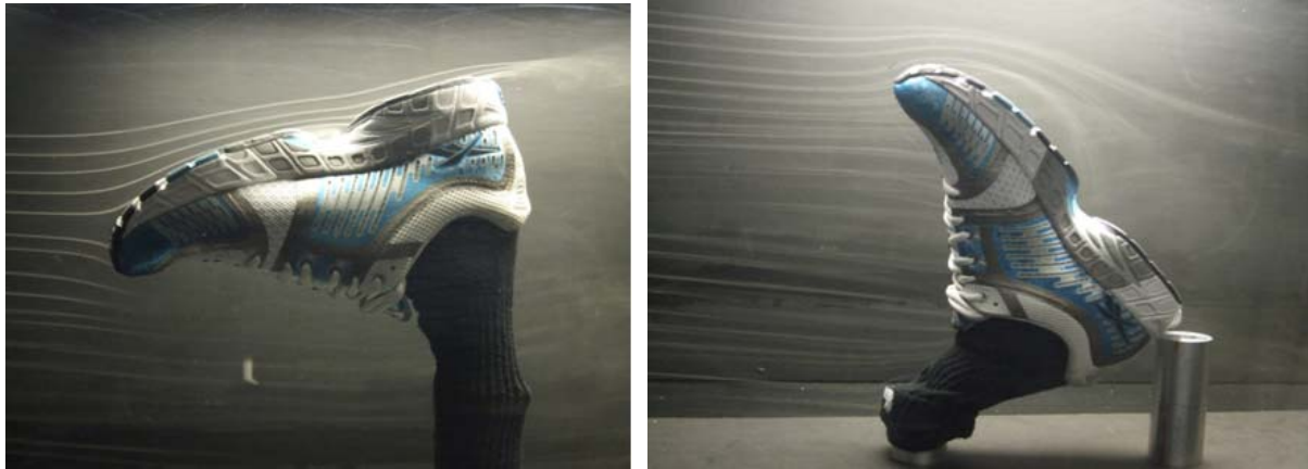
Fig. 6 Shoes at 10° and 50° in smoke tunnel
