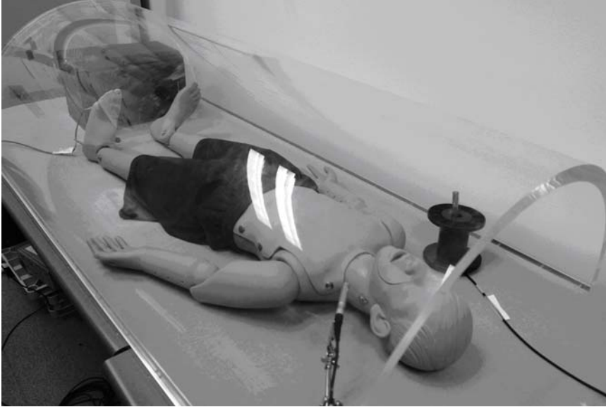
Fig. 8: Experiment 3 - Test-bed mimicking the MRI bore
