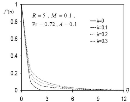
Figure 10: Velocity profiles for different values of mixed convection parameter  $\lambda$  at  $f_0 = 1.5$ .
