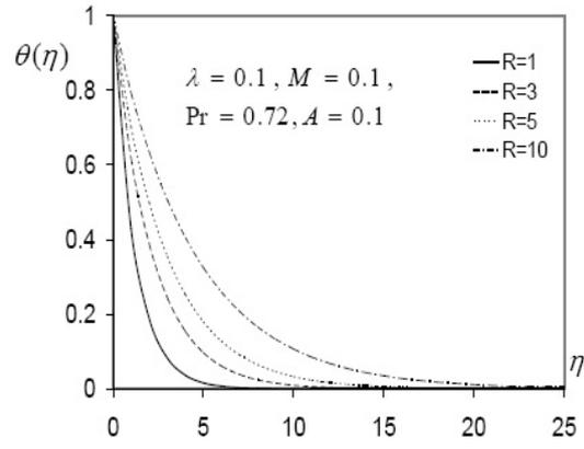
Figure 9: Temperature profiles for different values of radiation parameter  $R$  at  $f_0 = 1.5$ .
