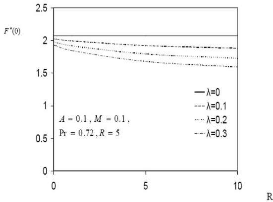
Figure 2: Variation of the skin friction coefficient as a function of radiation parameter R for various values of  $\lambda$  at  $f_0 = 1.5$ .
