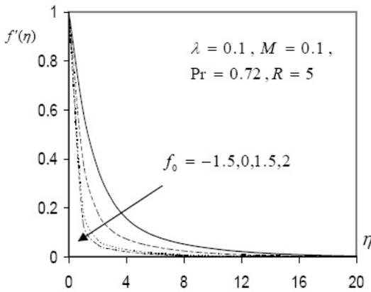
Figure 4: Velocity profiles for different values of suction/injection parameter at  $A = 0.1$ .
