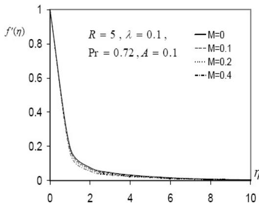
Figure 12: Velocity profiles for different values of magnetic parameter  $M$  at  $f_0 = 1.5$ .
