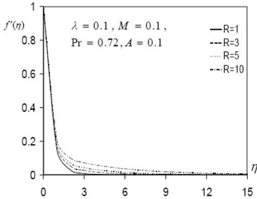
Figure 8: Velocity profiles for different values of radiation parameter  $R$  at  $f_0 = 1.5$ .
