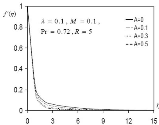
Figure 6: Velocity profiles for different values of unsteadiness parameter  $A$  at  $f_0 = 1.5$ .
