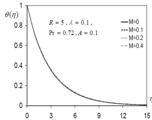
Figure 13: Temperature profiles for different values of magnetic parameter  $M$  at  $f_0 = 1.5$ .
