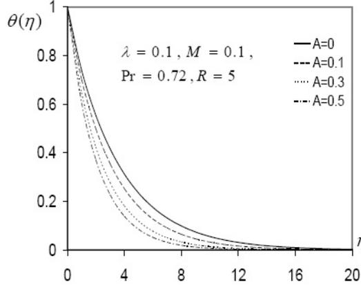
Figure 7: Temperature profiles for different values of unsteadiness parameter  $A$  at  $f_0 = 1.5$ .
