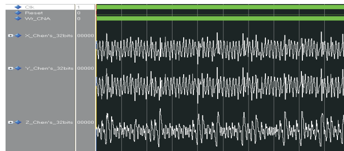
Figure 5: Simulation results of the Chen's chaotic generator ( x , y and z ), obtained by ModelSim.
