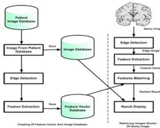
Fig. 3: The proposed shape image retrieval system
