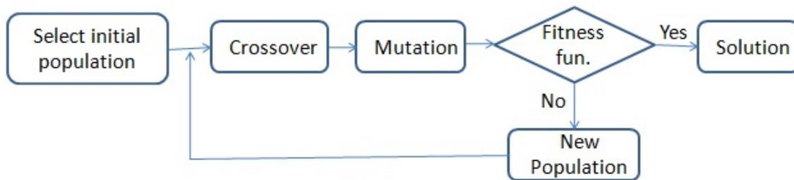
Figure 1: The structure of a simple genetic algorithm
