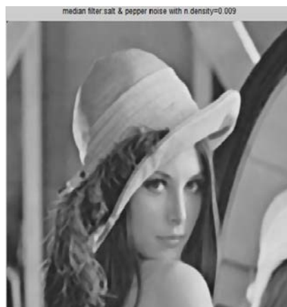
Fig. 18: De-noising by Median Filter for Salt & Pepper noise with noise density=0.009
