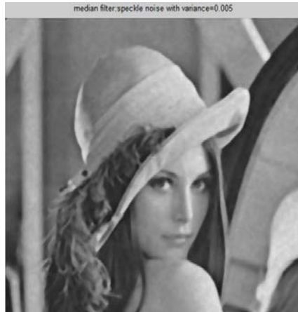
Fig. 13: De-noising by Median filter for Speckle noise with variance=0.005
