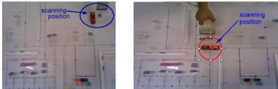
Fig. 10: Simulation of bar code scanning of an AGV at a certain position in the line.
