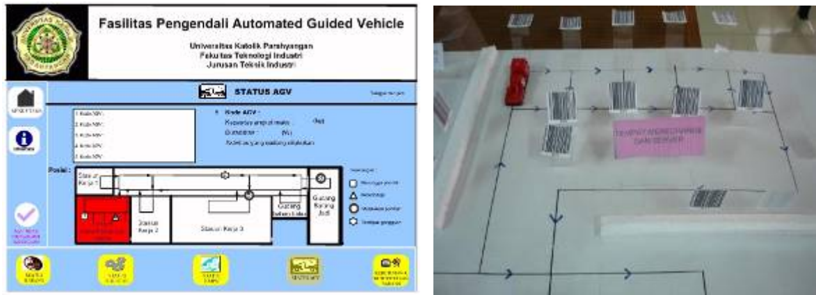
Fig. 7: (a) AGV controlling facility main menu, (b) AGV on the experimental setup (shop floor model).
