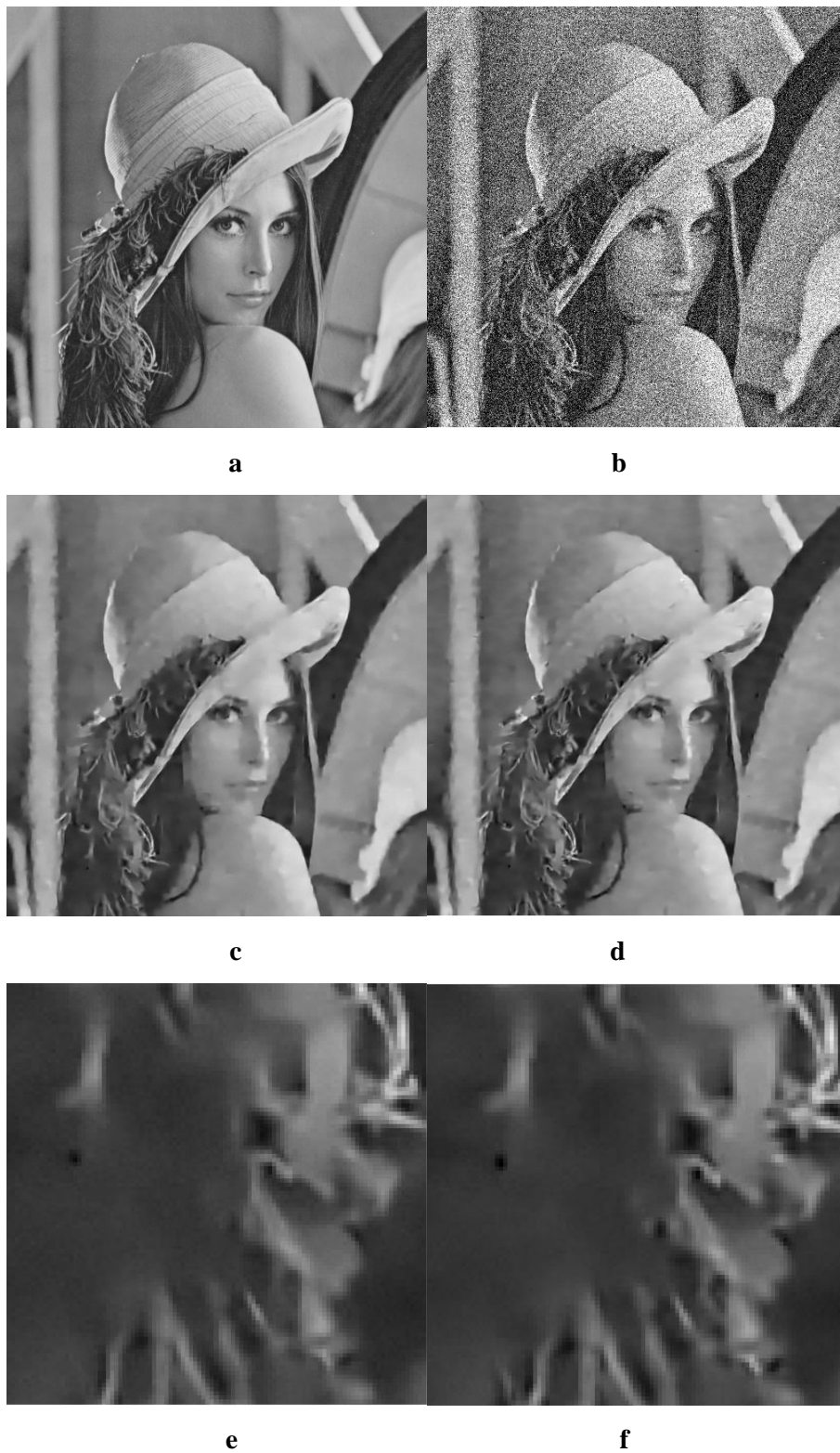
Figure2: Denoising results on 'lena' image with a standard variance \sigma = 50 . (a) Original image (b) Noisy image, (c) EPLL result (d), Proposed method, (e) EPLL enlarged partial result, (f) Proposed method enlarged partial result
