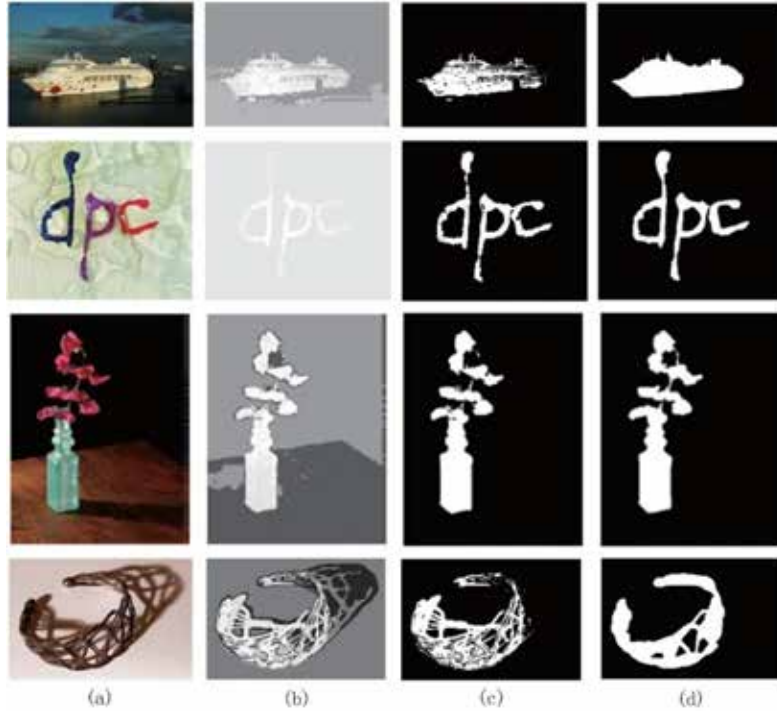
Figure 5: A demonstration extracting salient object. (a) The original image; (b) the saliency map; (c) the extracted and binarized salient object; (d) Ground True.
