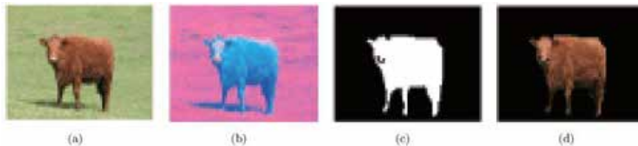
Figure 3: An example using MSRSG to detect and extract. (a) The original image; (b) the segmented image; (c) the binary image; (d) the salient object image.
