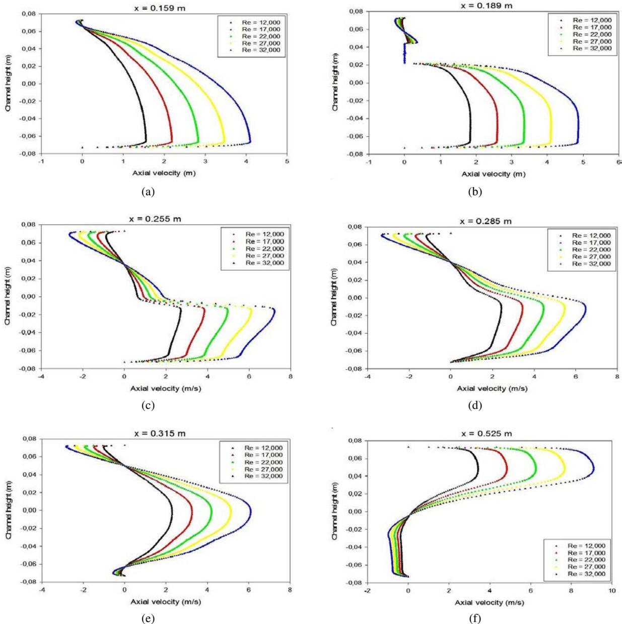
Fig. 8: Axial velocity profiles versus Reynolds number for different axial stations, (a)  $x = 0.159m$ , (b)  $x = 0.189m$ , (c)  $x = 0.255m$ , (d)  $x = 0.285m$ , (e)  $x = 0.315m$ , and (f)  $x = 0.525m$ .
