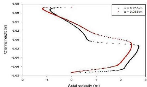
Fig. 5: Axial velocity profiles between the two 45° V-shaped baffles for  $Re = 12,000$
