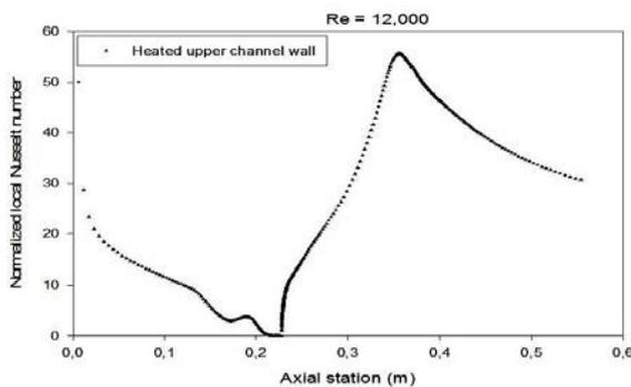
Fig. 10: Normalized local Nusselt number distribution along the heated upper channel wall length at  $Re = 12,000$ .
