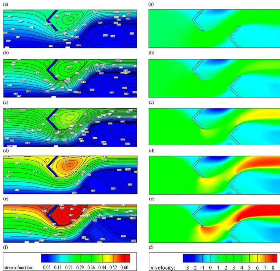
Fig. 3: Variation of streamlines and axial velocity fields with Reynolds number.
