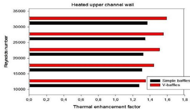
Fig. 14: Performance evaluation for both simple and V-baffles
