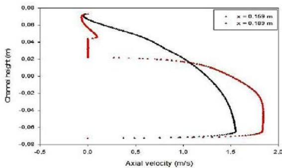
Fig. 4: Axial velocity profiles upstream of the first 45° V-shaped baffle for  $Re = 12,000$
