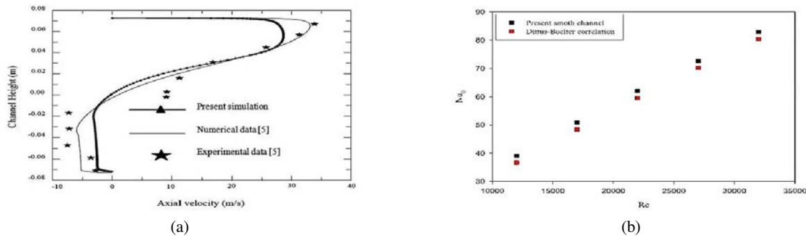
Fig. 2: Validation of (a) axial velocity profiles at  $x = 0.525$  m, and (b) smooth channel average Nusselt number at the heated upper channel wall, with reported data.
