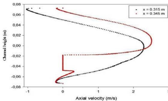
Fig. 6: Axial velocity profiles upstream of the second 45° V-baffle for  $Re = 12,000$
