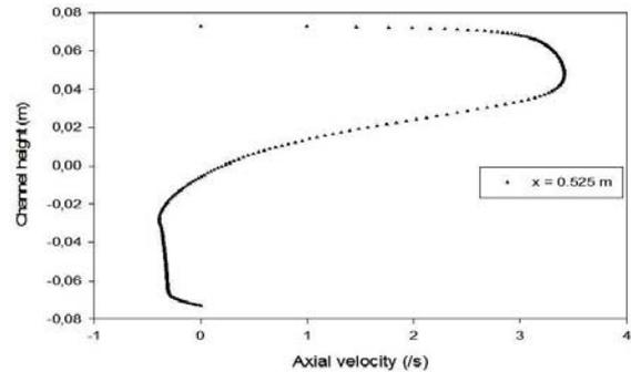
Fig. 7: Axial velocity profiles after the second 45° V-shaped, near the outlet for  $Re = 12,000$
