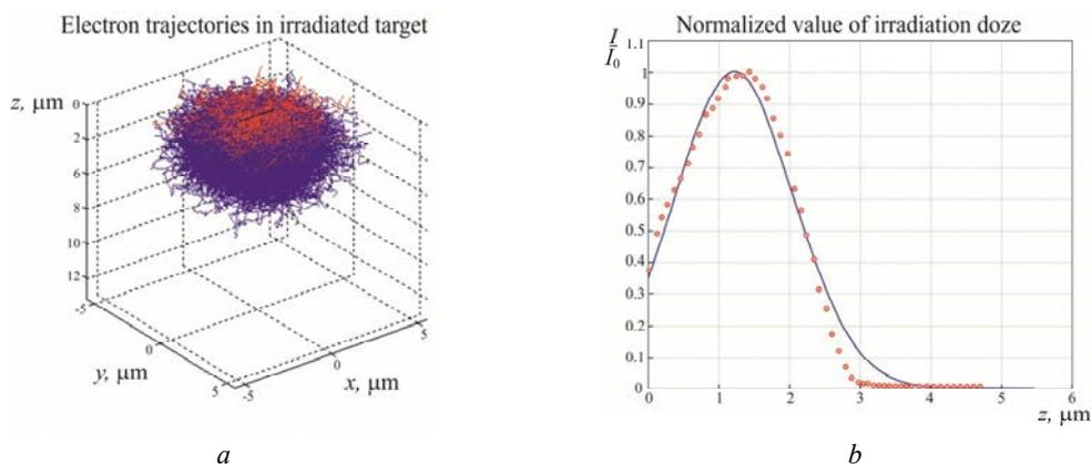
Fig. 2: The 3D-simulated electron trajectories –a, the accumulated irradiation dose in normalized units –b in TGS (at start beam energy  $E_0 = 15keV$ , number of electrons  $N = 5000$ , blue trajectories correspond to electrons injected into the sample, whereas red trajectories indicate backscattering electrons)
