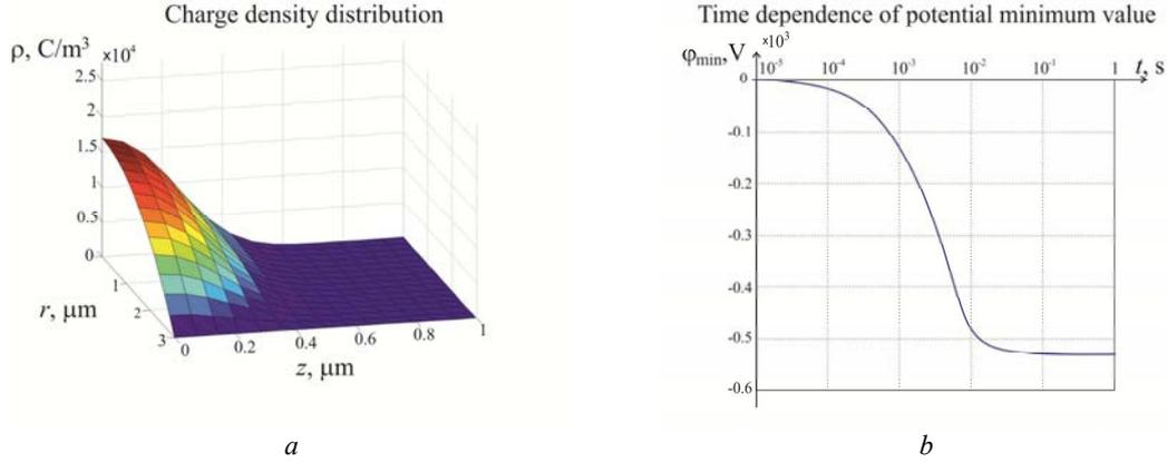
Fig. 3: The spatial distribution of charge density at time moment  $t^* = 5 \text{ ms}$  – a; time dependent variation of potential minimum value – b
