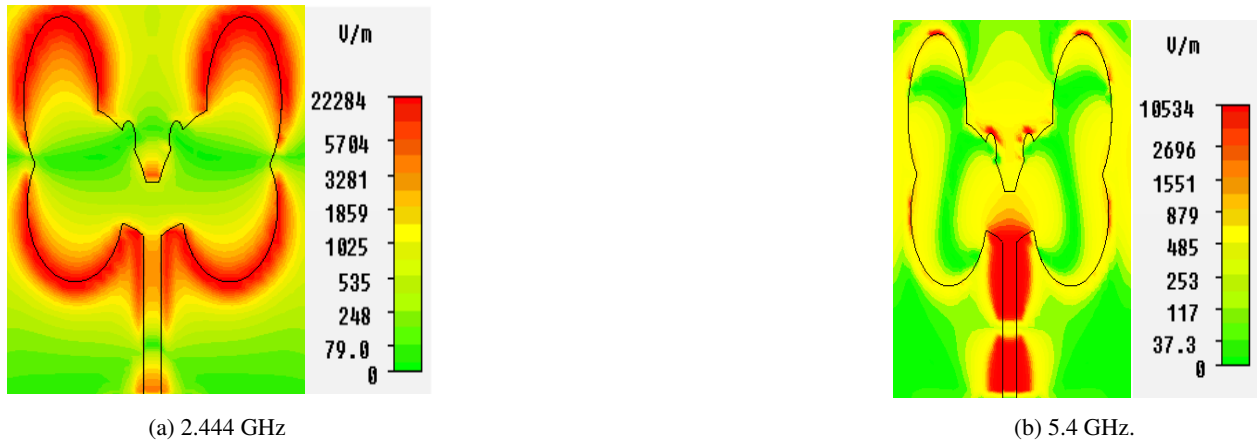
Fig. 6: E-fields radiated by traditional antenna
