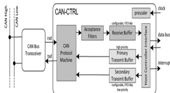
Fig. 1: Block diagram of CAN protocol
