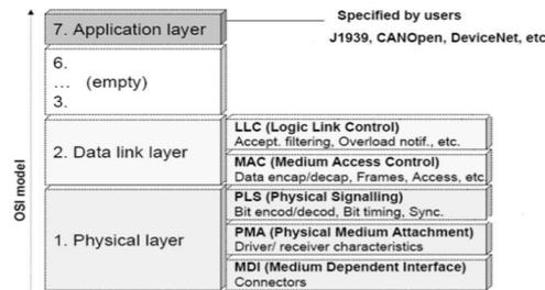
Fig. 3: The layered ISO 111898 standard architecture
