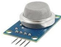
Fig. 8: MQ4 gas sensor
