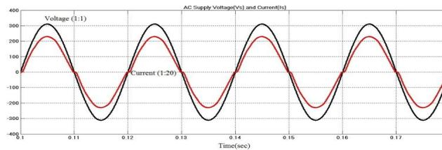
Fig. 13: Supply voltage and current waveforms in closed-loop operation
