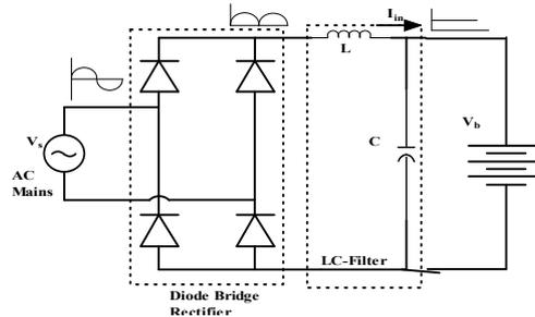
Fig. 1: Fundamental battery charging circuit diagram
