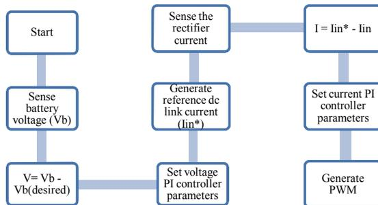
Fig. 11: Flow chart of buck-boost PFC converter control
