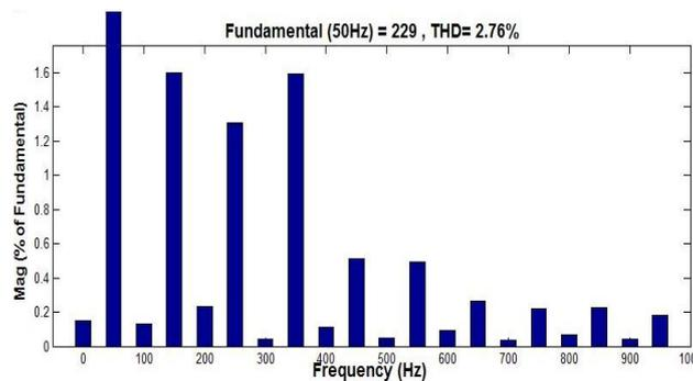
Fig. 14: THD spectrum of supply current in close loop control
