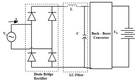
Fig. 4: Block diagram of battery charger with buck-boost converter in dc-link
