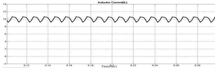
Fig. 12: Inductor current of buck-boost converter in closed-loop Operation
