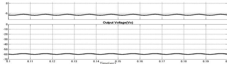
Fig. 8: Output current and voltage of buck-boost converter
