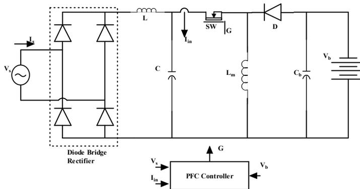
Fig. 10: Circuit of PFC charge controller in closed loop
