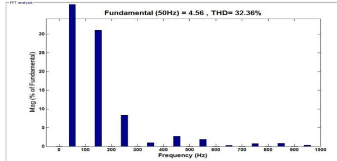
Fig. 7: THD spectrum of supply current
