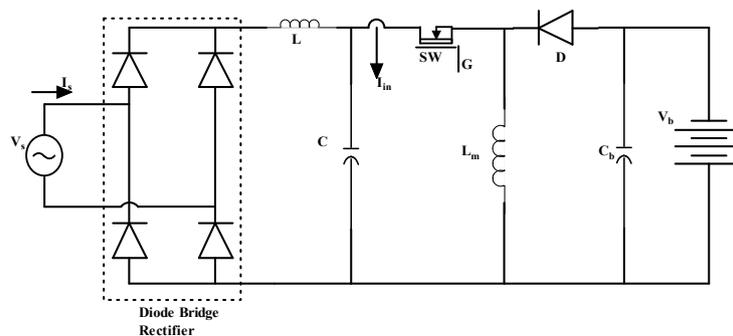
Fig. 5: Battery charging with buck-boost converter circuit in open-loop
