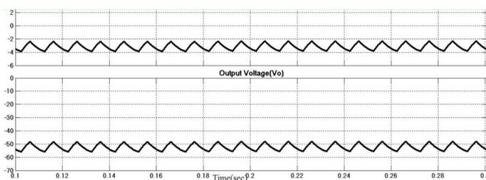
Fig. 15: Output current and voltage of buck-boost converter
