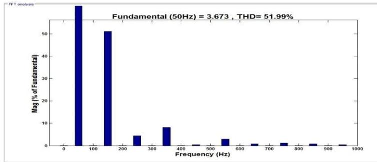
Fig. 3: THD spectrum of supply current
