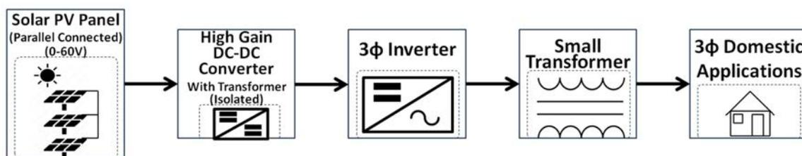
Fig. 1: Stand-alone PV system with isolated DC-DC converter
