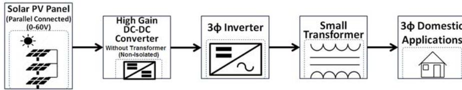
Fig. 2: Stand-alone PV system with non isolated DC-DC converter
