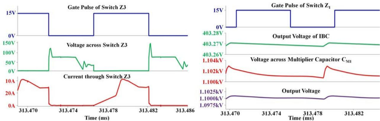
Fig. 8: (a): Voltage and Current Stress on Switch  $Z_3$  (b): Voltage across Capacitors at Various Stages
