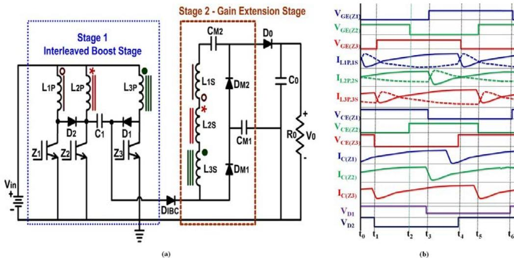
Fig. 3: (a) Proposed converter circuit (b) Characteristic Waveforms
