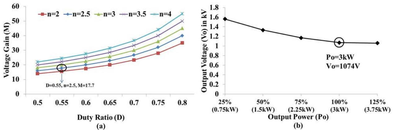
Fig. 5: (a): Voltage gain (M) Vs Duty cycle (D) (b): Output Voltage (V0) Vs Output Power (P0)
