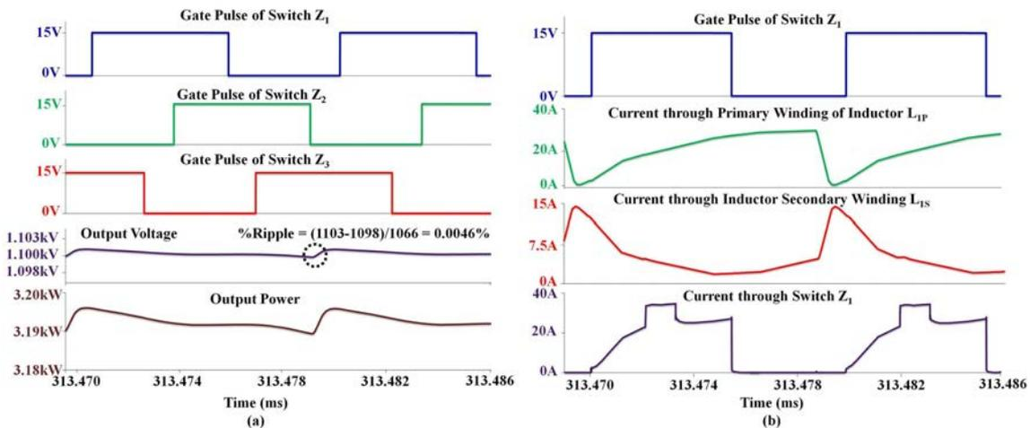
Fig. 6: (a): Gate pulses, output voltage and output power (b): Current through inductor  $L_2$  and switch  $Z_2$
