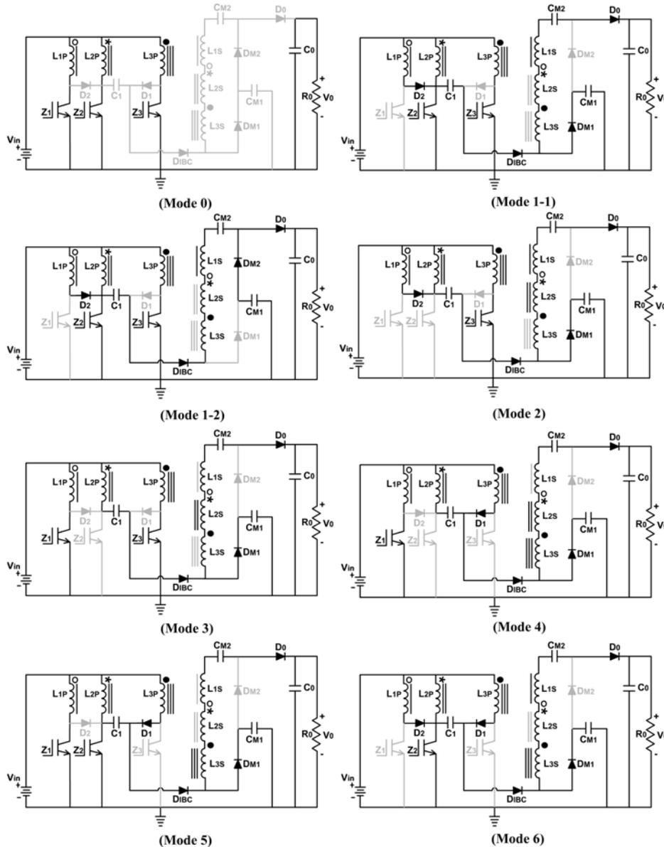
Fig. 4: Modes of operation of the proposed converter
