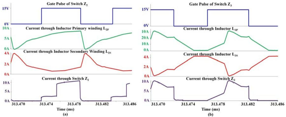
Fig. 7: (a): Current through Inductor L1 and Switch  $Z_1$  (b): Current through Inductor  $L_3$  and Switch  $Z_3$
