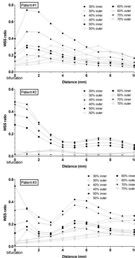
Fig. 5: Wall shear stress ratios at the inner wall and outer wall of the internal carotid artery (ICA) at the different degrees of stenosis
