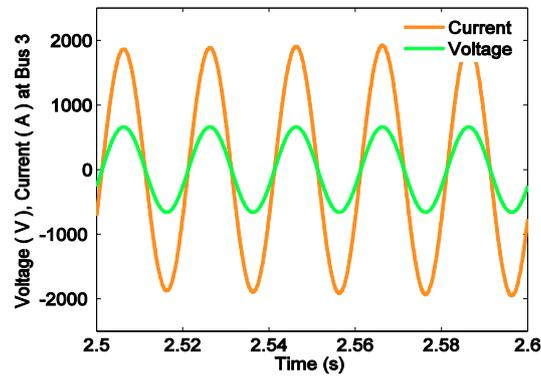
Fig. 15. The waveforms of three Phase current and voltage at Bus 3
