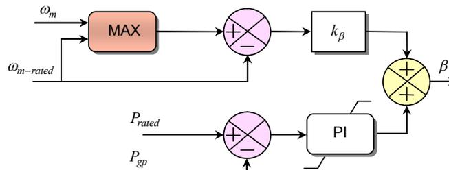
Fig. 2. WECS Pitch angle controller
