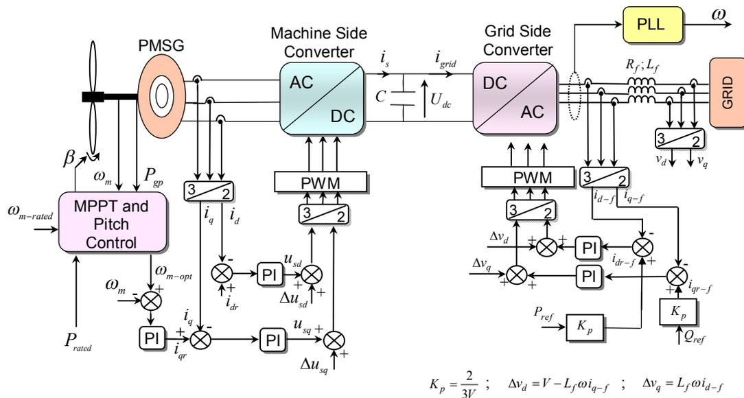
Fig. 3. Schematic of control strategy for VS-WECS based on the PMSG
