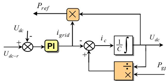
Fig. 5. Control of DC-bus voltage
