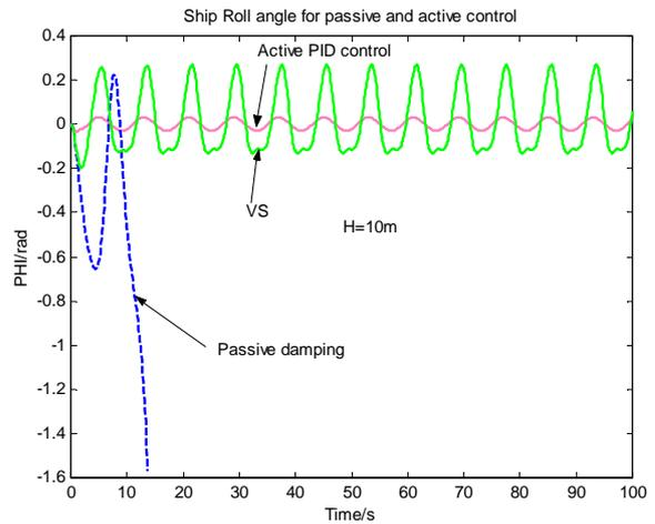
**Fig. 5.** Comparison of passive damping, elevon active control and Cycloidal propeller actuation for  $H = 10$  m
