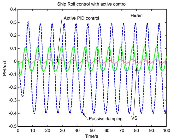
**Fig. 4.** Comparison of passive damping, elevon active control and Cycloidal propeller actuation for  $H = 5$  m
