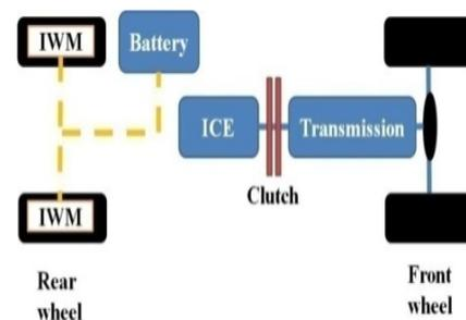
Fig. 2. Proposed parallel hybrid configuration
