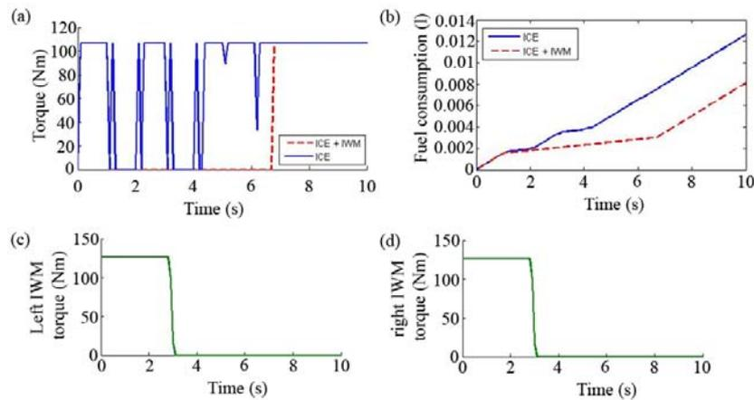
**Fig. 13.** Fuel consumption during cornering results (a) ICE torque comparison (b) Fuel use comparison (c) Left IWM torque (d) Right IWM torque
