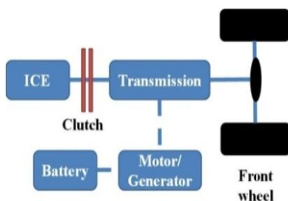
Fig. 1. Common parallel hybrid used by other researchers
