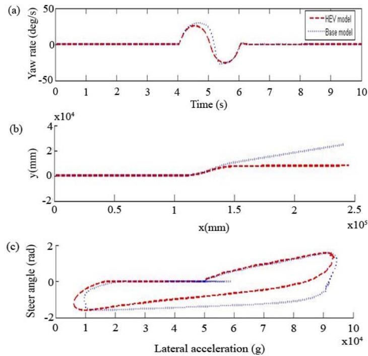
Fig. 9. Vehicle dynamics simulation results (a) Vehicle yaw rate (b) Vehicle path (c) Understeer gradient
