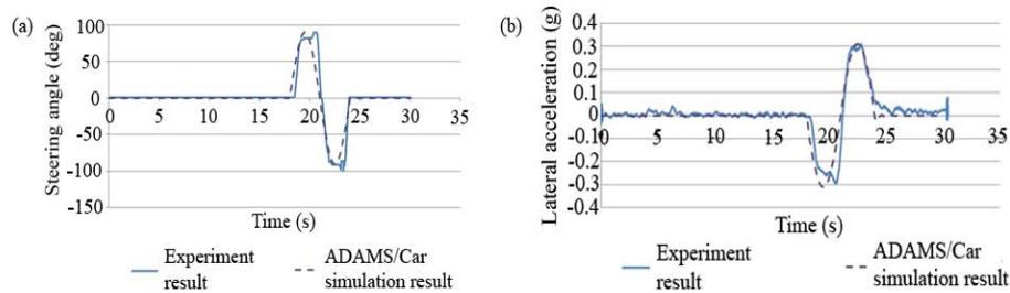
**Fig. 8.** Results for single lane change test (a) Steering wheel input (b) Lateral acceleration
