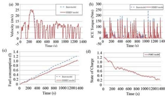
**Fig. 11.** Combined simulation results (a) Velocity profile comparison (b) ICE torque comparison (c) Fuel use comparison (d) SoC of HEV model
