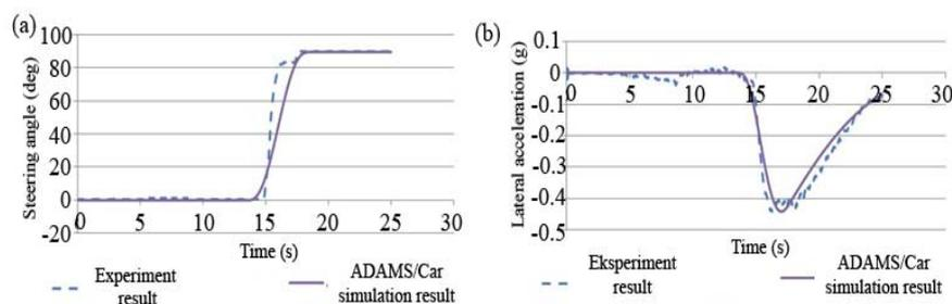
**Fig. 7.** Results for step steer test (a) Steering wheel input (b) Lateral acceleration
