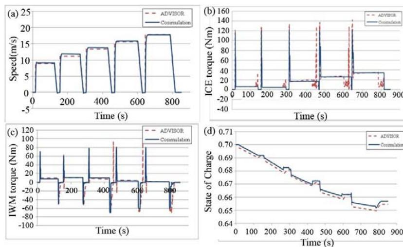
Fig. 10. Energy management simulation results (a) Velocity profile comparison (b) ICE torque comparison (c) IWM torque comparison (d) SoC comparison
