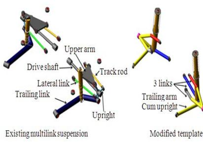
**Fig. 3.** Modification of existing multi-link suspension template
