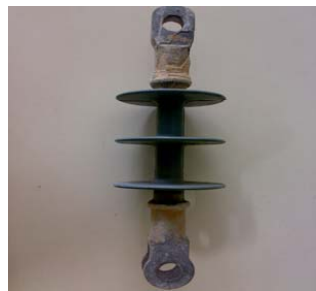
Fig. 1. Photograph of 11 kv silicon rubber insulator
