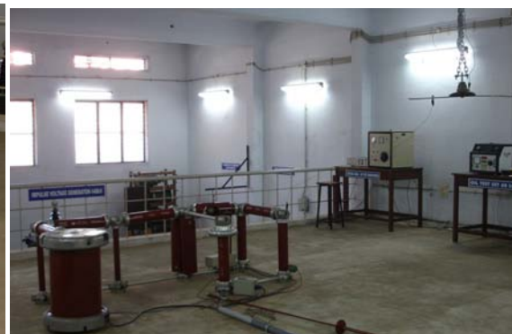
Fig. 6. Experimental setup for flash over testing of disc insulator
