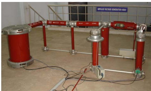
Fig. 5. Impulse voltage generator
