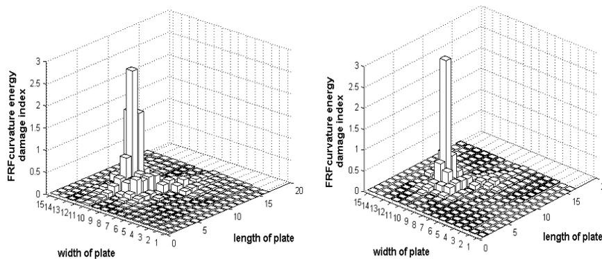
Fig. 4. FRF curvature energy damage index for a frequency range of 0-900 Hz. (a) Case 1 (b) Case 2
