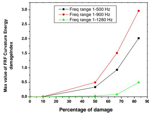
**Fig. 8.** Variation of percentage of damage versus maximum value of FRF curvature energy damage index for different frequency ranges
