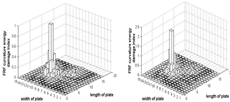
Fig. 3. FRF curvature energy damage index for a frequency range of 0-500 Hz. (a) Case 1 (b) Case 2
