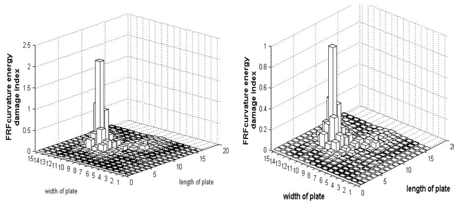
Fig. 6. FRF curvature energy damage index for a frequency range of 0-500 Hz. (a) Case 1 (b) Case 2
