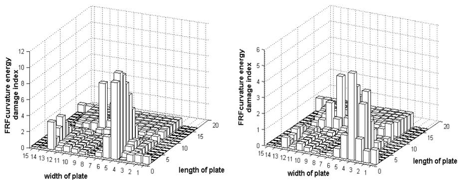
Fig. 5. FRF curvature energy damage index for a frequency range of 0-1280 Hz. (a) Case 1 (b) Case 2
