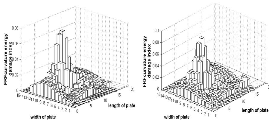
Fig. 7. FRF curvature energy damage index for a frequency range of 0-500 Hz. Case 1
