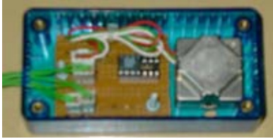
Fig. 3. Gyroscope CRS03 with temperature compensation
