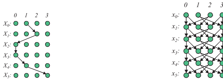
Fig. 5. The first 5 transition steps for MC simulation Fig. 6. The first 5 transition steps for the power method
